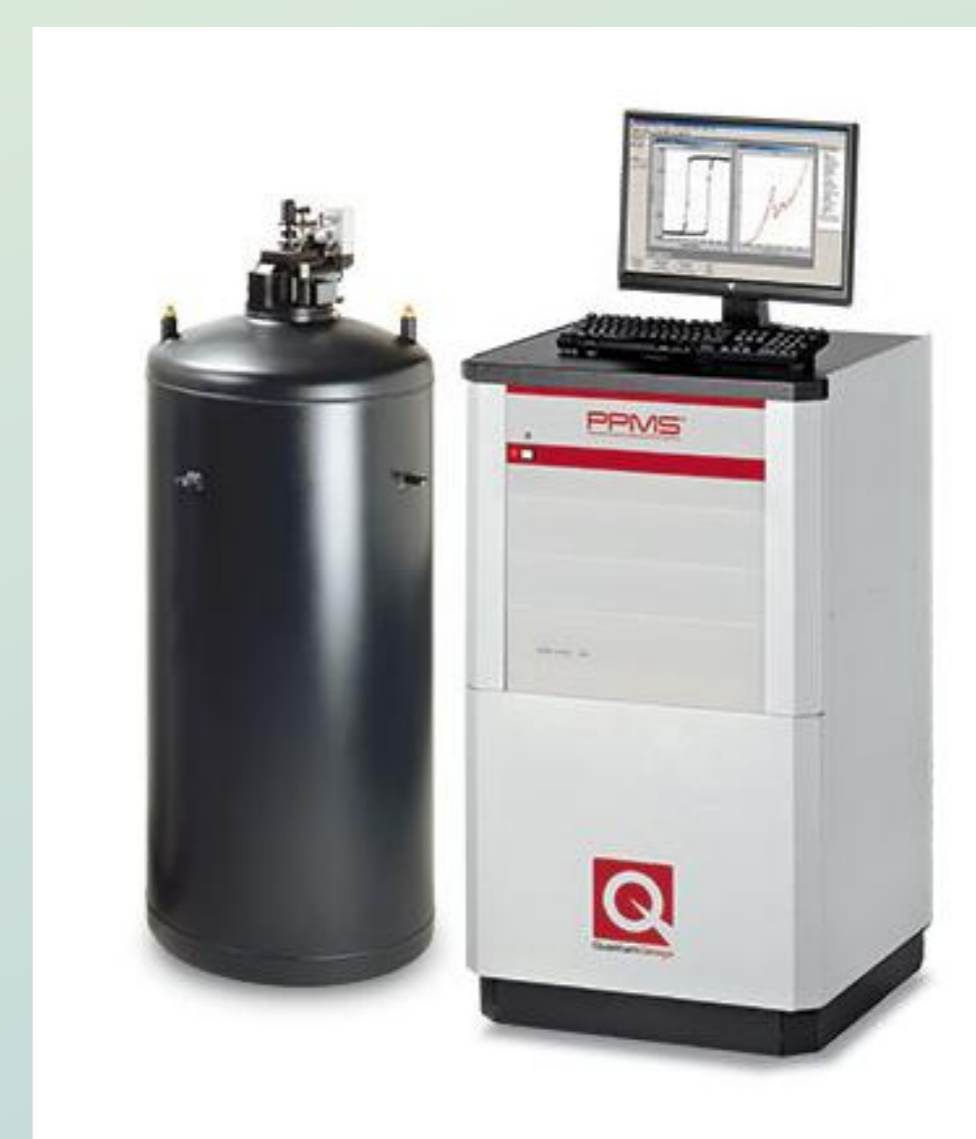
Fig. 4 The specific heat was determined using the method of thermal relaxation on a commercially available Physical Properties Measurement System (PPMS, Quantum Design Inc.)
